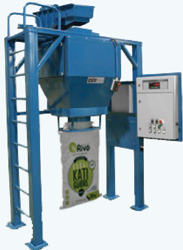
Figure 9. Packaging unit to be used in vermicompost facility
